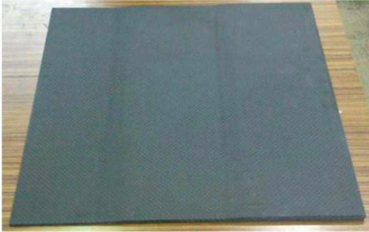
Figure 11. Apparatus of cured CFRP panel with thickness variation.
